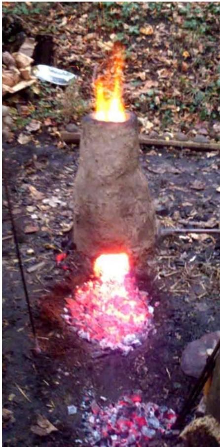
This picture shows the smelting of iron in a bloomery. The bloomery is clay, and it's filled with iron ore, charcoal, and a flux. What comes out when the furnace is tapped and cooled is a spongy mass of iron, which has to be reheated and hammered by a blacksmith to turn it into usable iron.
